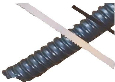
The conduit has to be held firmly by hand and a fine teeth saw is to be used to cut it. It has to be cut at right angles and any burrs should be trimmed either with a file or a sharp pair of strips.
